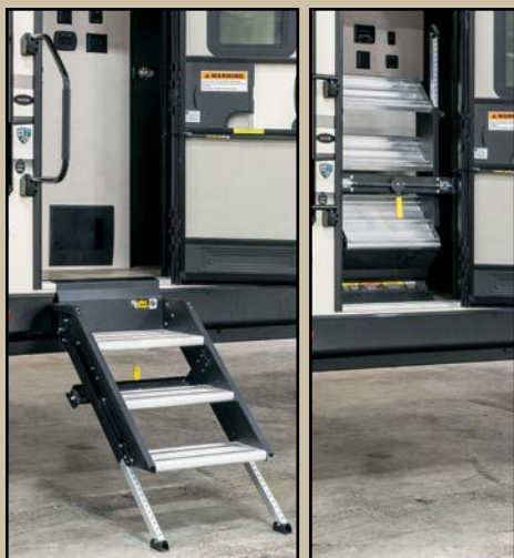
Standard flip-up entry step with large folding grab handle provide solid footing, and folds up in one easy motion.
