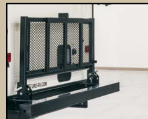
Optional flip-up storage rack, for cargo or two bicycles, folds flush when not in use.
