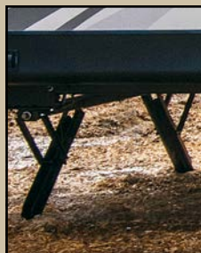
Four power jacks, each with its own independent motor.
