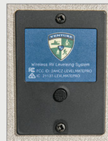
Sonic's LevelMate wireless leveling system calculates a perfect level position without time-consuming guesswork. (Sonic & Sonic Lite)
